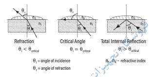
In the **MA871**, light from an LED passes through a prism in contact with the sample. An image sensor determines the critical angle at which the light is no longer refracted through the sample. The **MA871** automatically applies temperature compensation to the measurement and converts the refractive index of the sample to sucrose concentration in units of percent (by weight) Brix.
