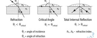
In the MA873, light from an LED passes through a prism in contact with the sample. An image sensor determines the critical angle at which the light is no longer refracted through the sample. The MA873 automatically applies temperature compensation to the measurement and converts the refractive index of the sample to Glucose concentration in units of percent (by weight).
