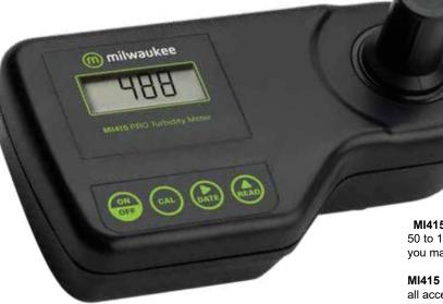
Turbidity refers to the concentration of undissolved, suspended particles present in a liquid. Turbidity is a measure of the clarity of a sample. For potable water applications turbidity is a good indicator of water quality.
