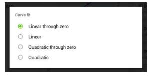
The curve statistics are also displayed for the curve fit chosen. For example if the curve fit is y = mx+c the curve statistics displayed will be the gradient of the line (m), constant (c) and correlation coefficient ( $r^2$ ).
