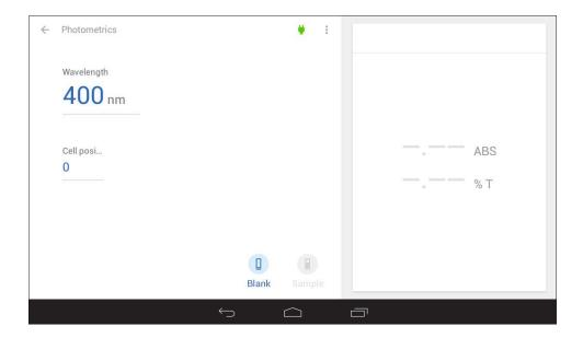
Set up the required measurement parameters. Insert the cuvette containing the blank solution into turret position 0 followed by the cuvettes containing the samples into turret positions 1 to 7 and close the instrument lid.
