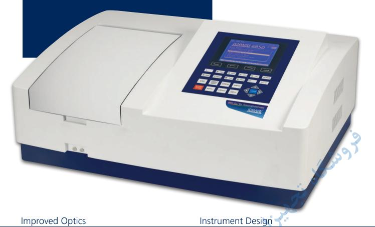
Model 6850 covers the UV/visible wavelength range from 190 to 1100nm, with a variable spectral bandwidth, ranging from 5nm down to 0.5nm, using tungsten halogen and deuterium light sources. The range of bandwidths available allows a balance between resolution, accuracy and data precision to be maximised depending on the application; therefore providing a flexible platform to conform to multiple regulatory agencies for a variety of applications, all with one spectrophotometer.
