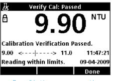
Be confident in your measurement by running the quick and easy Verify Cal function using the included 10 NTU StablCal primary standard.
