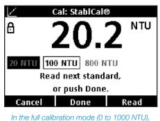
the text-based, assisted calibration feature walks you through clear and easy steps, and verifies the accuracy of your calibration automatically. This on-screen assistance eliminates the need for a manual and provides assurance that your calibration is complete and valid.
