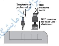
The temperature probe is used in conjunction with the pH electrode to utilize the meter's ATC capability, but it can also be used independently to take temperature measurements. If the probe is disconnected, the temperature can be set manually using the arrow keys.
