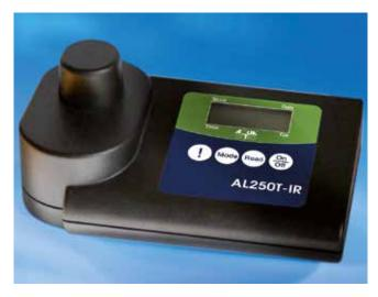
The compact AQUALYTIC® infrared turbidity measuring instruments AL255T-IR & AL250T-IR for fast and accurate on-site analysis. It is measured as provided in EN ISO 7027, the scattered light at an angle of 90 °.
