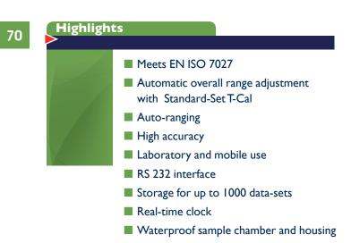
Turbidity is measured according to EN ISO 7027 by nephelometric means (90° scattered light). The infra-red light-source permits measurement of coloured and colour-free samples. The automatic measurement range detection facility (Autorange) enables direct turbidity measurement from 0.01 to 1100 NTU with an accuracy of  $\pm 2\%$  up to 500 NTU and  $\pm 3\%$  thereafter.
