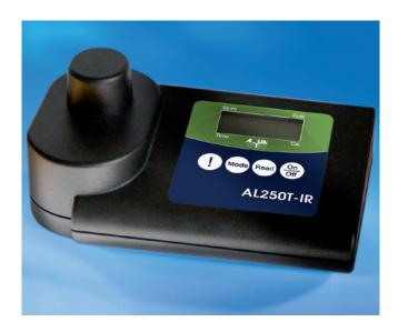
The compact AQUALYTIC® infrared turbidity meter AL250T-IR is designed to allow fast, precise on-site testing. The unit measures the scattered light at an angle of 90°, as stipulated in EN ISO 7027.
